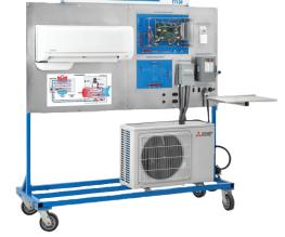
The T7130 was designed to include transparent housings and pipes with LED illumination that allows learners to see inside the system. Learners will also
