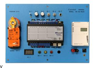
level, users interact via PC software to connect with web-based configurations where they test and communicate with BAS/DDC field controllers. Using the Sedona Framework, users can create a basic DDC program that includes the three fundamental elements of controls: inputs, logic, and outputs. Offering students hands-on experience with DDC, this benchtop unit features a Contemporary Controls Bc022 controller and (2) BACnet discoverable devices including a Bellimo Actuator and Senva wall setter.
